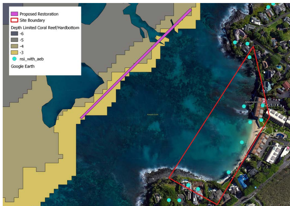
Figure 1H. Map showing the Kahana Sunset CR4 project site. The area predicted to receive the most risk reduction benefits from the restoration project is outlined in red. The individual structure annual expected benefit provided by the addition of 1m in reef height is summarized by the teal dots. The isolated area considered feasible for restoration based on depth from 2 m to 7 m and existing coral reef or hardbottom benthos is represented in shades of yellow to blue. The proposed restoration project site is represented in purple.
