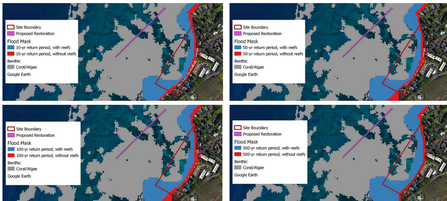
Figure 2H. Maps showing the extent of flooding from multiple storm return periods for the with reefs (blue) and without reefs (red) scenarios at the Kahana Sunset site.
