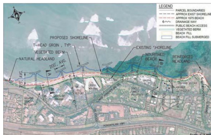
Figure 1D. A rendering of the proposed T-groin and beach restoration project to enhance and restore the beach and reduce erosion in the Kahana project area.
