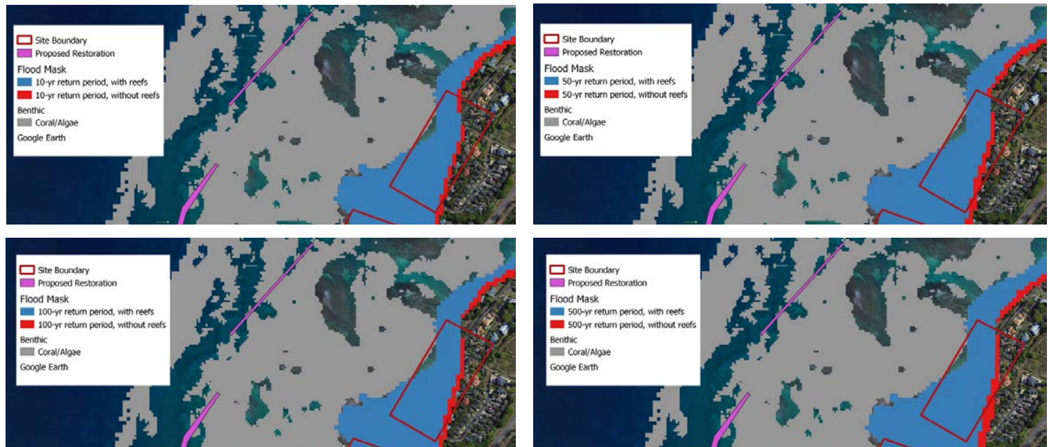
Figure 2J. Maps showing the extent of flooding from multiple storm return periods for the with reefs (blue) and without reefs (red) scenarios at the Kahanaiki Gulch site.
