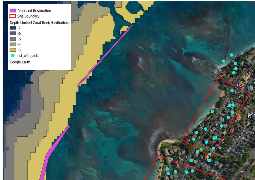
Figure 1J. Map showing the Kahanaiki Gulch CR4 project site. The area predicted to receive the most risk reduction benefits from the restoration project is outlined in red. The individual structure annual expected benefit provided by the addition of 1m in reef height is summarized by the teal dots. The isolated area considered feasible for restoration based on depth from 2 m to 7 m and existing coral reef or hardbottom benthos is represented in shades of yellow to blue. The proposed restoration project site is represented in purple.
