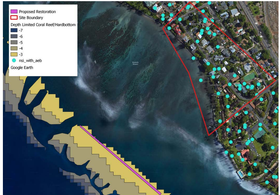
Figure 1N. Map showing the Kauaula Stream CR4 project site. The area predicted to receive the most risk reduction benefits from the restoration project is outlined in red. The individual structure annual expected benefit provided by the addition of 1m in reef height is summarized by the teal dots. The isolated area considered feasible for restoration based on depth from 2 m to 7 m and existing coral reef or hardbottom benthos is represented in shades of yellow to blue. The proposed restoration project site is represented in purple.
