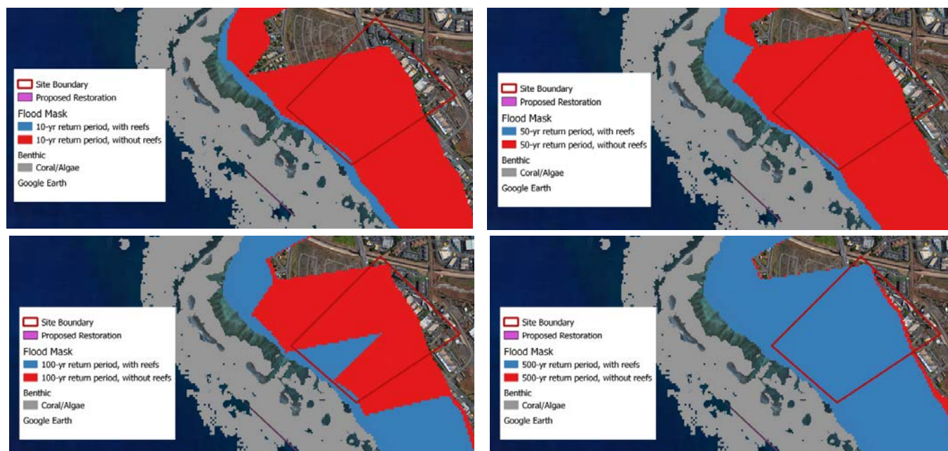
Figure 2C. Maps showing the extent of flooding from multiple storm return periods for the with reefs (blue) and without reefs (red) scenarios at the Lahaina site.
