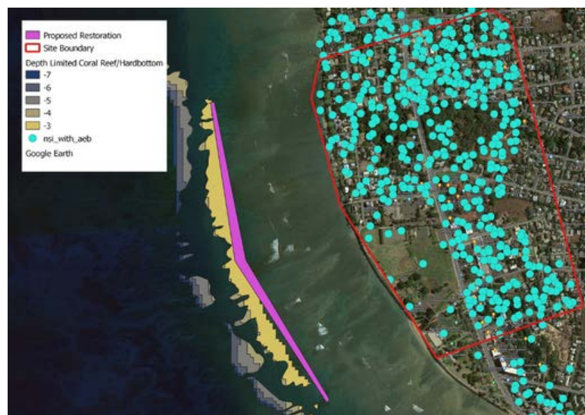
Figure 1E. Map showing the South Kihei CR4 project site. The area predicted to receive the most risk reduction benefits from the restoration project is outlined in red. The individual structure annual expected benefit provided by the addition of 1m in reef height is summarized by the teal dots. The isolated area considered feasible for restoration based on depth from 2 m to 7 m and existing coral reef or hardbottom benthos is represented in shades of yellow to blue. The proposed restoration project site is represented in purple.
