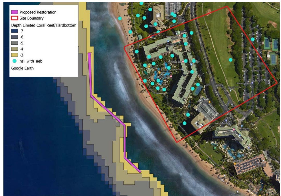
Figure 1G. Map showing the Ka'anapali Marriott CR4 project site. The area predicted to receive the most risk reduction benefits from the restoration project is outlined in red. The individual structure annual expected benefit provided by the addition of 1m in reef height is summarized by the teal dots. The isolated area considered feasible for restoration based on depth from 2 m to 7 m and existing coral reef or hardbottom benthos is represented in shades of yellow to blue. The proposed restoration project site is represented in purple.
