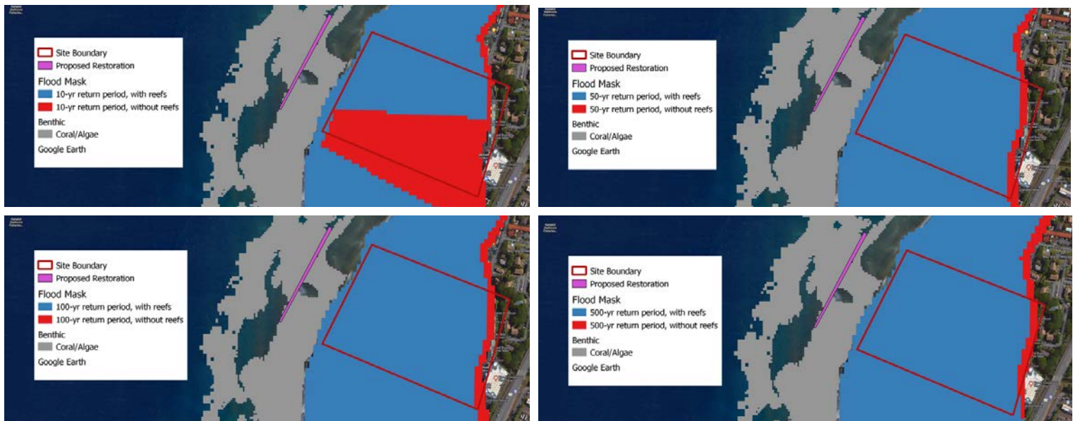
Figure 2A. Maps showing the extent of flooding from multiple storm return periods for the with reefs (blue) and without reefs (red) scenarios at the Ka'anapali Beach Club site.
