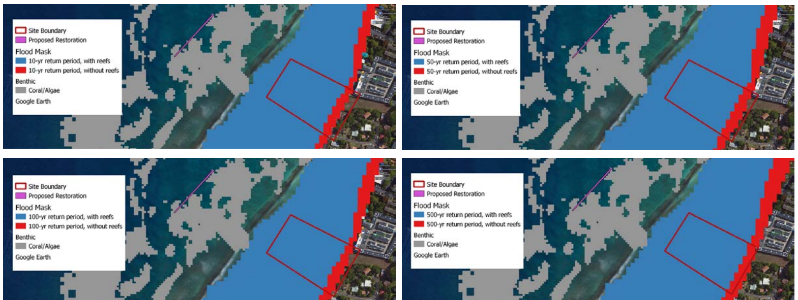
Figure 2L. Maps showing the extent of flooding from multiple storm return periods for the with reefs (blue) and without reefs (red) scenarios at the Maui Sands site.
