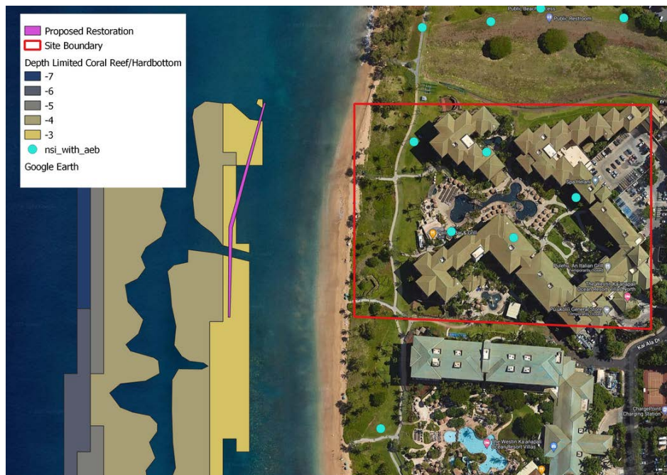
Figure 1M. Map showing the Westin Ka'anapali CR4 project site. The area predicted to receive the most risk reduction benefits from the restoration project is outlined in red. The individual structure annual expected benefit provided by the addition of 1m in reef height is summarized by the teal dots. The isolated area considered feasible for restoration based on depth from 2 m to 7 m and existing coral reef or hardbottom benthos is represented in shades of yellow to blue. The proposed restoration project site is represented in purple.
