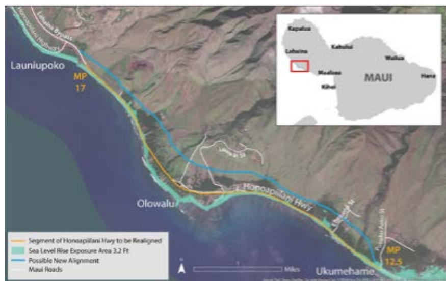
Figure 10. A preliminary figure from HI DOT showing the proposed realignment of the Honoapiʻilani Highway (Route 30).
