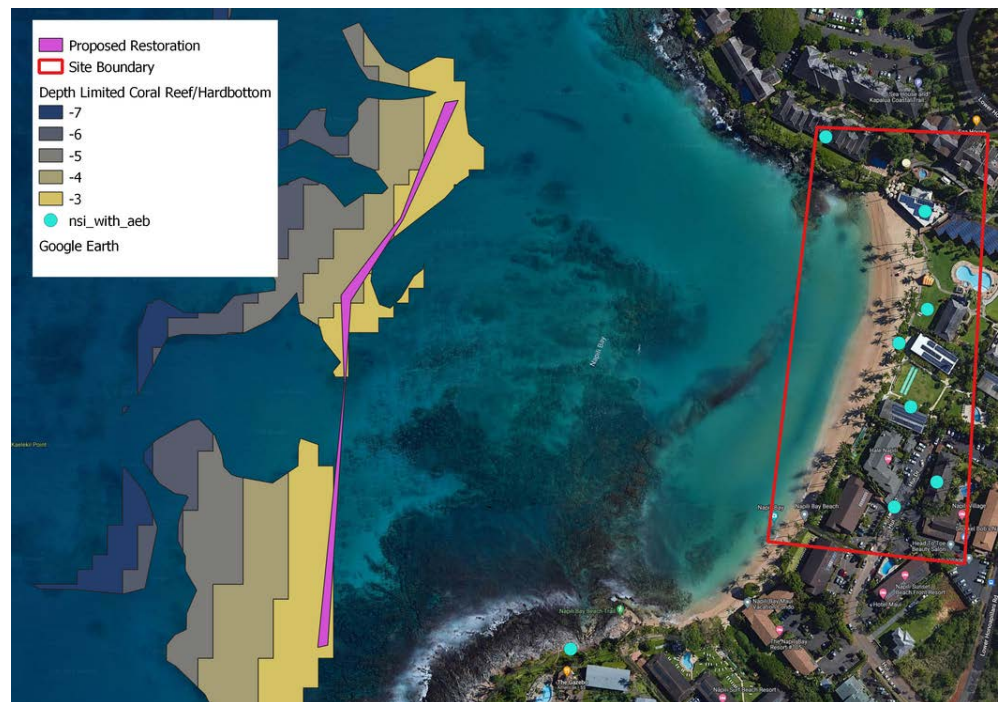
Figure 1I.. Map showing the Napili Bay CR4 project site. The area predicted to receive the most risk reduction benefits from the restoration project is outlined in red. The individual structure annual expected benefit provided by the addition of 1m in reef height is summarized by the teal dots. The isolated area considered feasible for restoration based on depth from 2 m to 7 m and existing coral reef or hardbottom benthos is represented in shades of yellow to blue. The proposed restoration project site is represented in purple.
