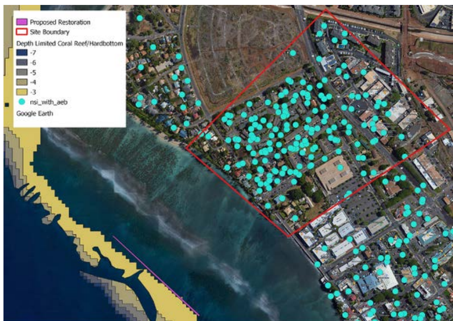
Figure 1C. Map showing the Lahaina CR4 project site. The area predicted to receive the most risk reduction benefits from the restoration project is outlined in red. The individual structure annual expected benefit provided by the addition of 1m in reef height is summarized by the teal dots. The isolated area considered feasible for restoration based on depth from 2 m to 7 m and existing coral reef or hardbottom benthos is represented in shades of yellow to blue. The proposed restoration project site is represented in purple.
