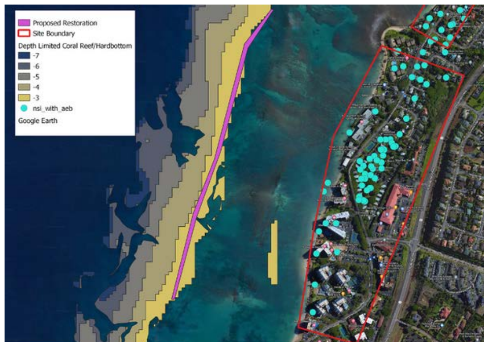
Figure 2D. Map showing the Kahana CR4 project site. The area predicted to receive the most risk reduction benefits from the restoration project is outlined in red. The individual structure annual expected benefit provided by the addition of 1m in reef height is summarized by the teal dots. The isolated area considered feasible for restoration based on depth from 2 m to 7 m and existing coral reef or hardbottom benthos is represented in shades of yellow to blue. The proposed restoration project site is represented in purple.
