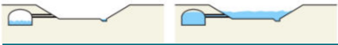
© DISEÑOARQUITECTURA.CL: Left: Underground stormwater channel with low water level. Right: After heavy rain when the maximum vault capacity is exceeded, and the water floods the park.
