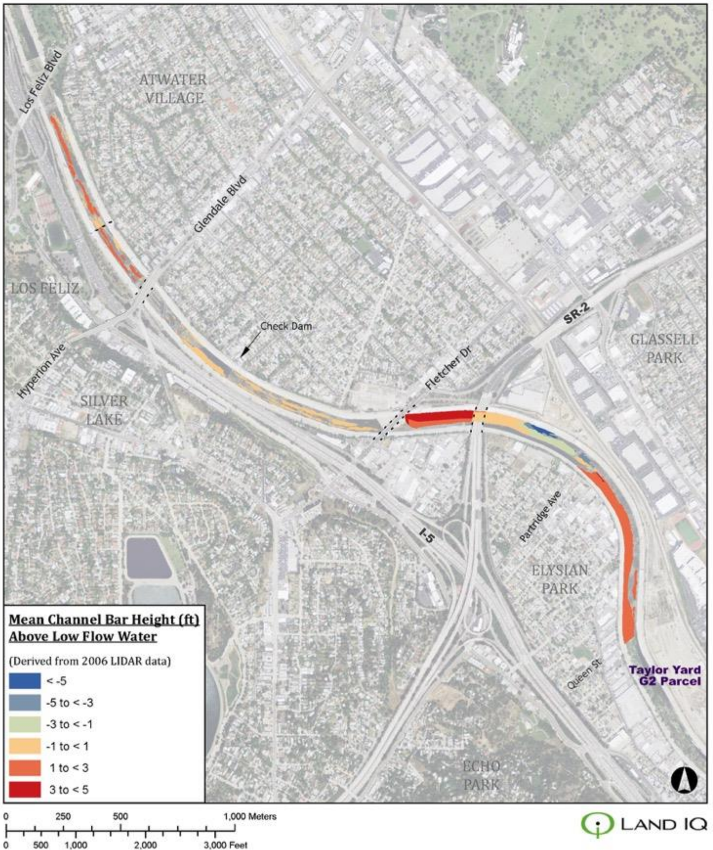
Figure 3-19 Mean channel bar height above low flow Los Angeles River water in the Elysian Valley.
