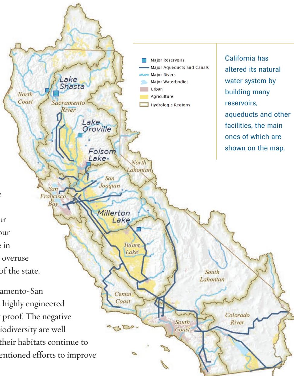
California has altered its natural water system by building many reservoirs, aqueducts and other facilities, the main ones of which are shown on the map.
