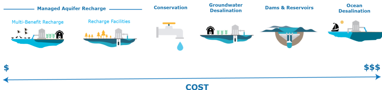
Figure 2. Water supply cost comparison, with the cost per unit of water increasing left to right (Modified from [2]. Data sources: Dynamic Recharge [3]; On-Farm Recharge [4]; Recharge Facilities [5]; Conservation [6]; Groundwater Desalination [7]; Dams & Reservoirs [8]; Ocean Desalination [9].
